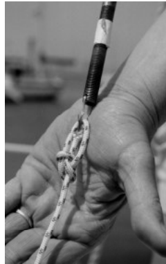
connecting swage stud to messenger line
