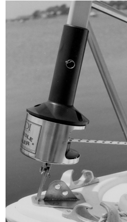
Furler w/ luff support pin installed
