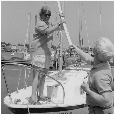
pushing extrusion up forestay
