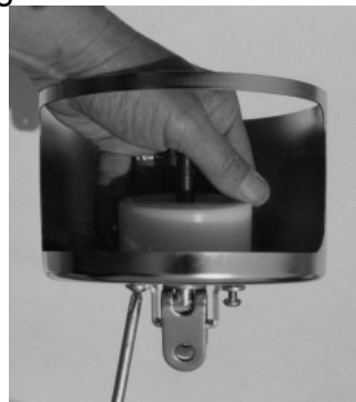
Assembling cup, bearing, and antirotation strap
